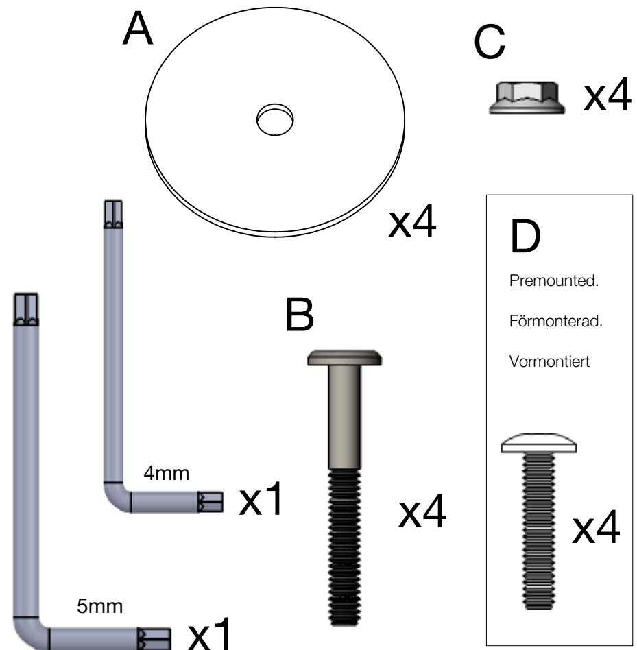
Unmount the swivel plate at the bottom of the seat by removing the four bolts "D". Put the wooden frame together and bolt it to the swivel plate with bolt "B", plastic washer "A" and nut "C". Remount the plate to the bottom of the seat.
